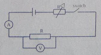
A battery, voltmeter, ammeter, rheostat and a resistance R are connected in a circuit as shown.
