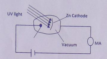
A zn cathode was enclosed in an evacuated tube as shown. When the cathode was irradiated with ultra violet radiation, the ammeter gave a reading. Explain why the ammeter gave.
