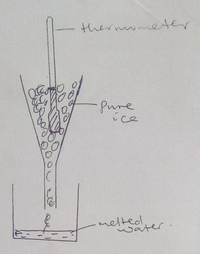
The bulb of the thermometer is inserted into ice in a funnel.
