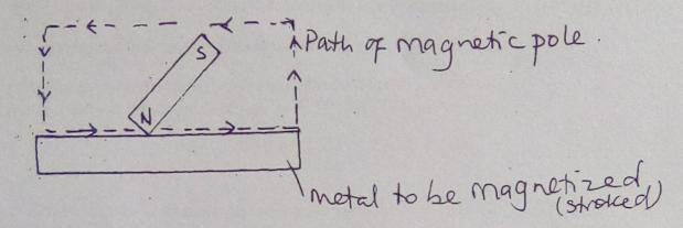
One pole of a bar magnet is moved (stroked) along the surface of the metal brand at the end it is lifted high off the bar. It is brought to the starting point to start a fresh cycle as shown by the path.
