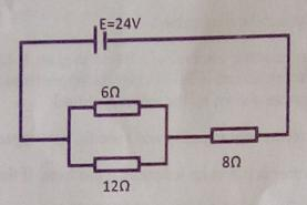
A battery of emf 24V and negligible internal resistance is connected to resistors of  $6\Omega$ ,
